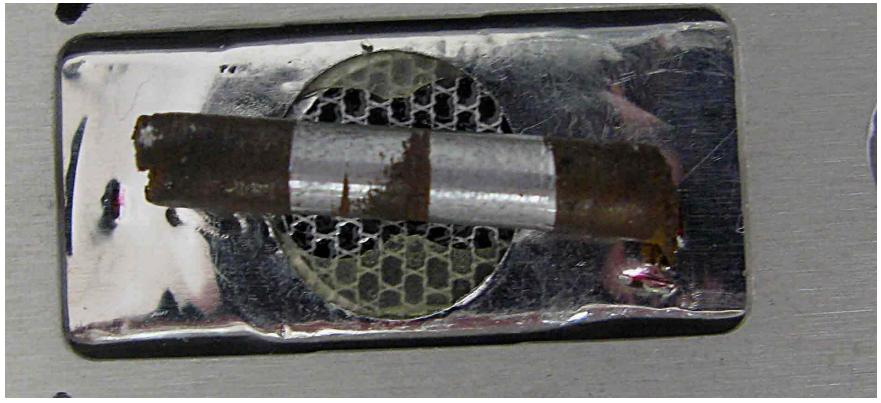
Above is the photograph of the rivet sitting on the instrument after the center section was machine .001" The side facing the XRF instrument has no dark corrosion present. The dark area in the center of the machined portion is because the rivet had a gouge on visible side so the machining process did not remove the corrosion in this location.
